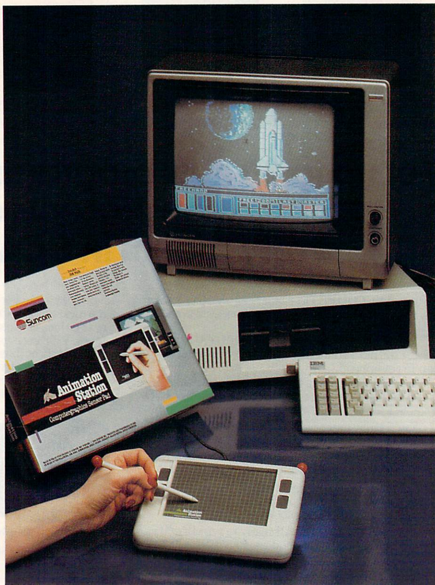
Animation Station, a graphics tablet designed by Suncom, offers a number of colors and textures for drawings like this.
