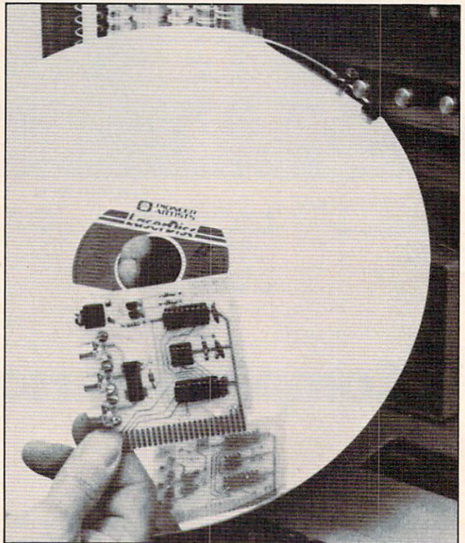
Anthro-Digital, Inc.'s Omniscan LaserDisc interface for use with an Apple computer and appropriate videodisc systems.
