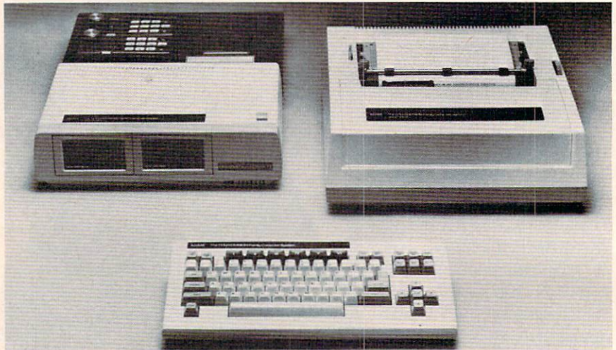
This version of the Adam converts the ColecoVision videogame machine into the computer system. It is functionally identical to the regular Adam.
