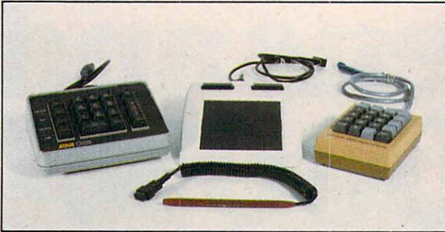
Light pens, touch tablets, and numeric keypads provide alternative ways of entering data into your computer.
