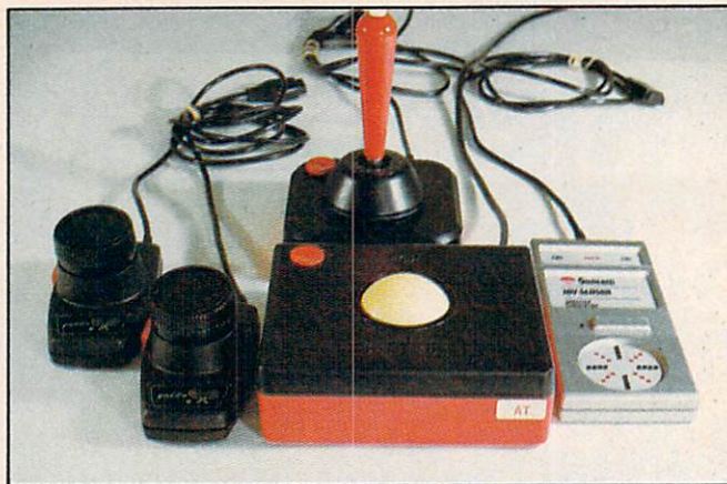
Game controllers come in a variety of styles, each of which has a different "feel." Shown here are paddles, a joystick, a trackball, and a pressure-sensitive controller.
