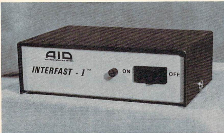
The Interfast-I is a programmable printer interface for Atari computers.
