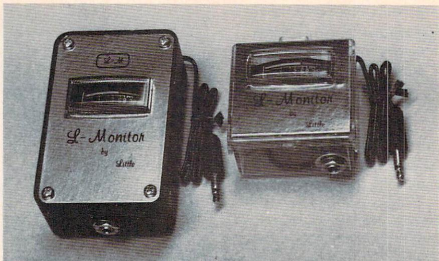
The L-Monitor, a microammeter used to improve transfer of data to or from cassette tape, comes in an assembled version, left, or in kit form.
