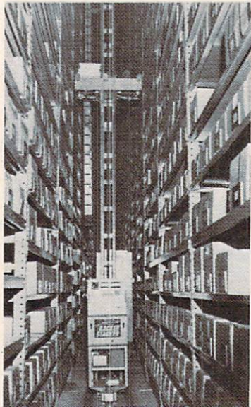
Figure 2: A crane, as seen from the front of an aisle, with its bed halfway up its mast
