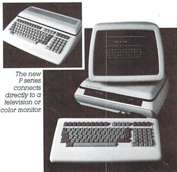
Commodore's B series features a tilt/swivel display and detachable keyboard.
