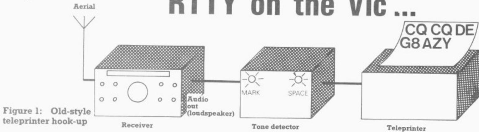
Figure 1: Old-style teleprinter hook-up
