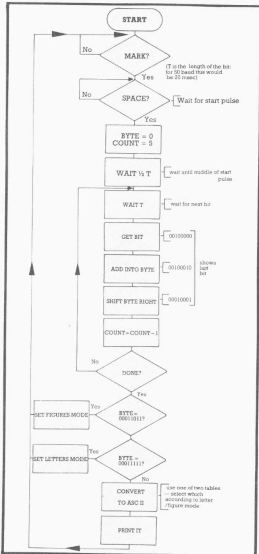
Figure 5: Simple flowchart for assembling and printing RTTY
