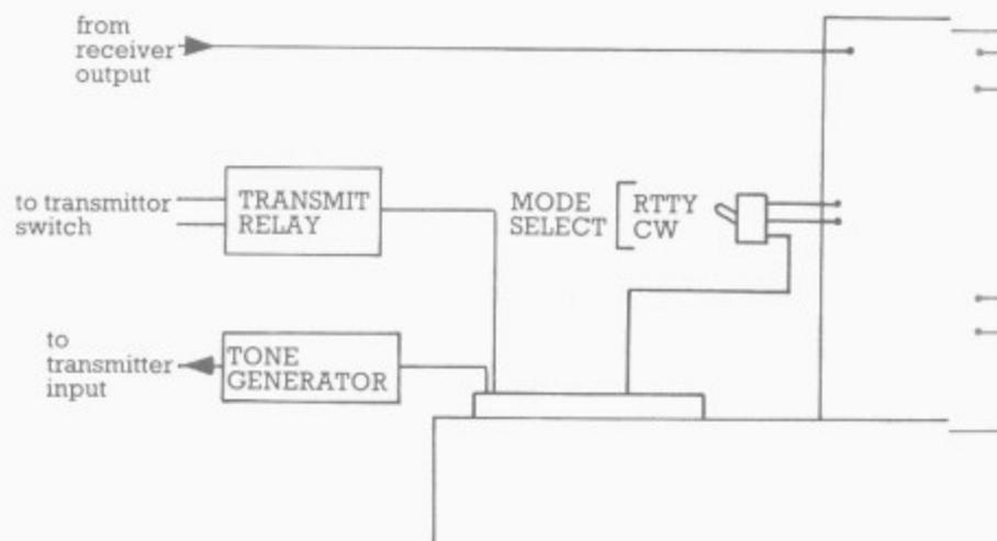
**Figure 6: Connections to TDK-20**
