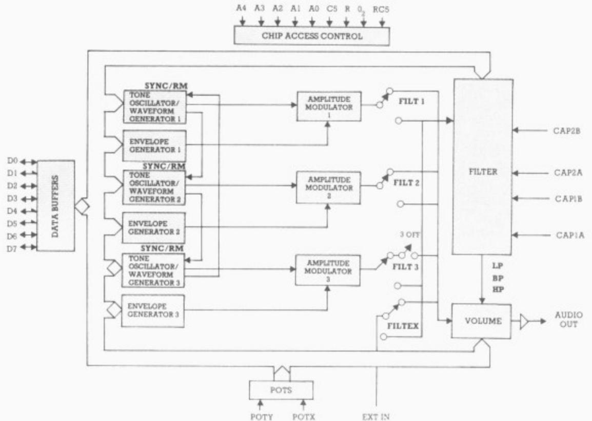
Figure 1: Block diagram of the SID
