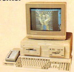
The Amiga 500 Command Center is now available from Ketek, Inc. to house your Amiga 500 drives. The Command Center can accommodate two 3.5-inch external drives or one 3.5-inch drive and a 20 or 30MB hard drive. The unit features a built-in cooling fan, surge suppression, noise filter and five-outlet power strip. The Amiga 500 Command Center retails for \$179.95. For more information contact: Ketek, Inc., P.O. Box 203, Oakdale, IA 52319. Or call: (800) 626-4582.
