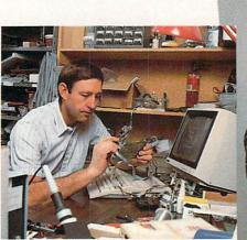
Final test and inspection of B100 interface using another B100.
