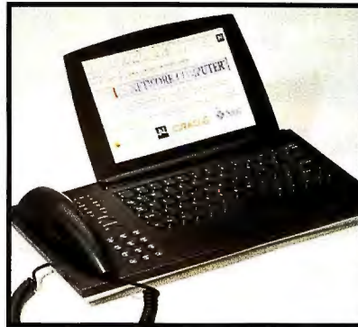
One of Oracle's four reference designs integrates a phone with an NC.
