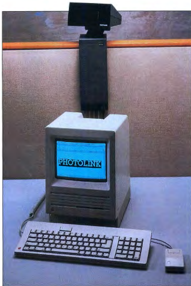
Each Photolink transceiver replaces a strand of LocalTalk cabling.
