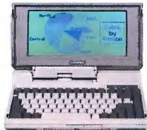
T1200HB: 10.8 lbs, 9.54MHz 80C86, 20MB hard disk, 1MB RAM, includes 384KB LIM-EMS. Removable/rechargeable battery pack.
