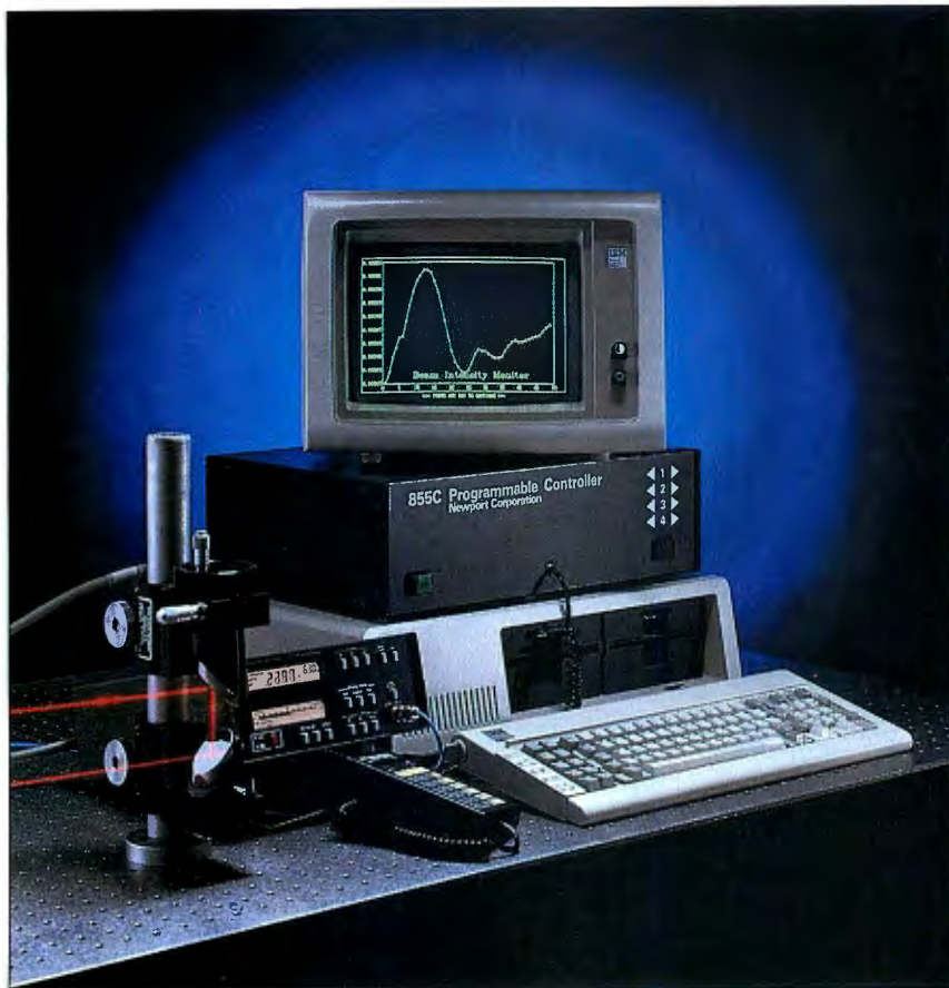
Photo 3: National Instruments software, controlling instrumentation for testing lasers. Notice the power meter and stage-positioning system integrated with an IBM PC under the control of LabWindows. The CRT display shows the laser-beam intensity. (Photo courtesy of Newport Corp.)
