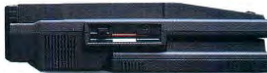
T5100: 16MHz 80386 microprocessor, 40 or 100MB hard disk, 2MB RAM expandable to 4MB. 14.6 lbs. Built-in EGA display with high resolution gas plasma screen.
