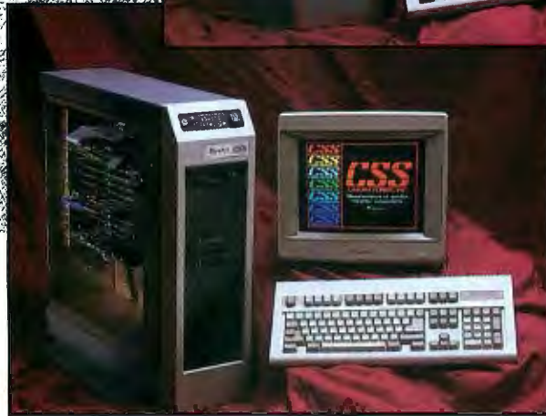
The MaxSys 386T (lower photo) and 386MT (upper photo) feature 12 slots to provide the systems with expandability.
