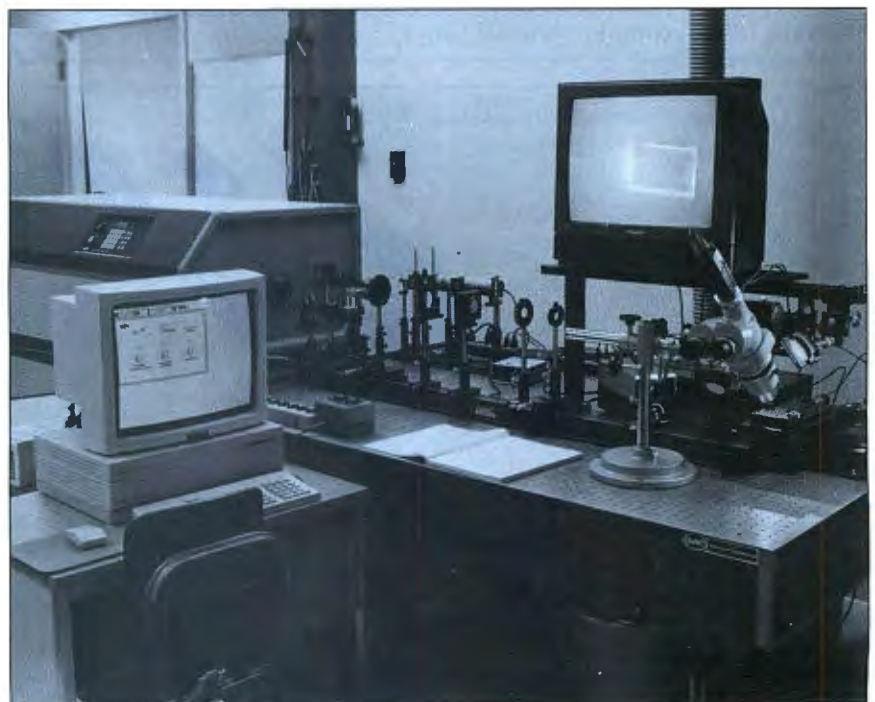
Photo 2: An excimer laser interfaced with a CAD system, and the same laser controlled by a Mac II under LabView. (Photo courtesy of Questek, Inc.)
