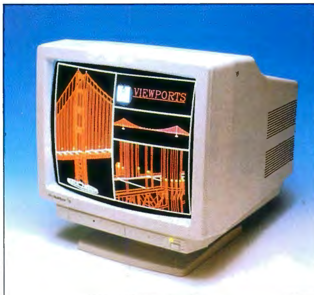
NEC's MultiSync 5D supports a variety of graphics modes, including VGA, SuperVGA, 8514/A, and Apple Mac II standards.
