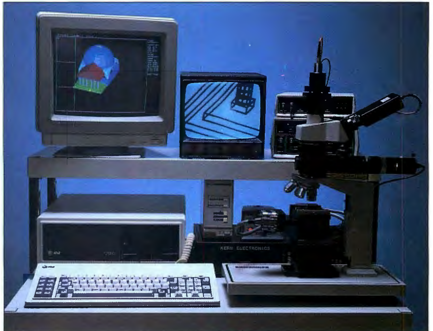
Photo 1: A Q-switched, diode-pumped, neodymium yttrium-aluminum-garnet laser from Spectra-Physics, attached to a microscope. Under control of the AT&T PC 6300, a CAD Design 3 image is being scribed onto a coated plate. The two monitors show the CAD image (in color) and a section of the scribed image (in black and white). Nicknamed the "Laser Blade," this system is unique in that the diode laser-beam pump light is transported from a power-supply box to the neodymium YAG laser head via an optical fiber. This results in a very small, pencil-size laser head that you can attach directly to the microscope. (Photo courtesy of W. Scarvie, Spectra-Physics, Inc.)
