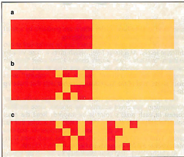
Figure 1: (a) Two adjacent blocks of color sharing a hard boundary. (b) The boundary in (a) has been softened with yellow-filled airbrush. (Each square equals one pixel.) (c) In this case, the hard boundary in (a) has been softened by smudging (i.e., by swapping pixels).
