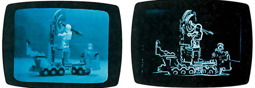
Photo 8: Edge detection with ImageWise. The image in (a) is processed through Edge, Multiply, and Thresh to produce (b).
