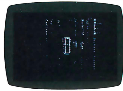
Photo 7: Here, I use the Thresh program to remove background noise from the image in photo 6b. The missing IC in 5b now stands out clearly.
