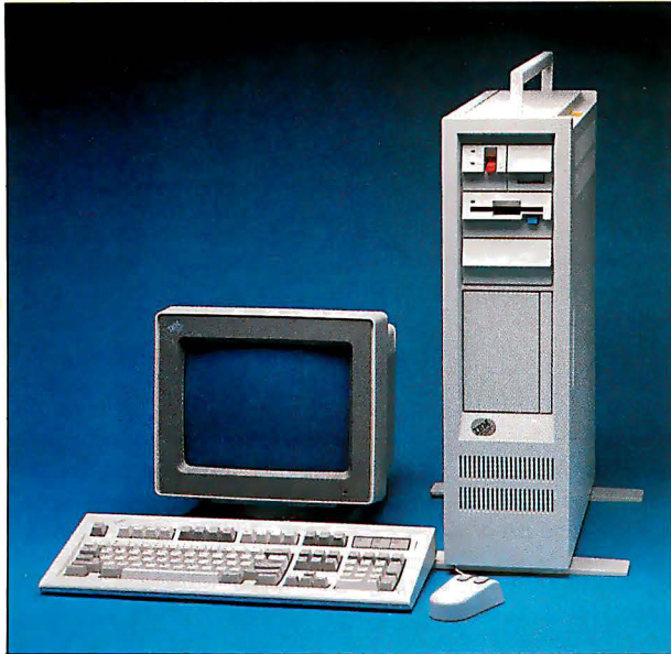
Photo A: The Model 60 with the 8503 monochrome monitor. The Model 60 is much larger than the Model 50; in fact, it stands on the floor beside your desk.
