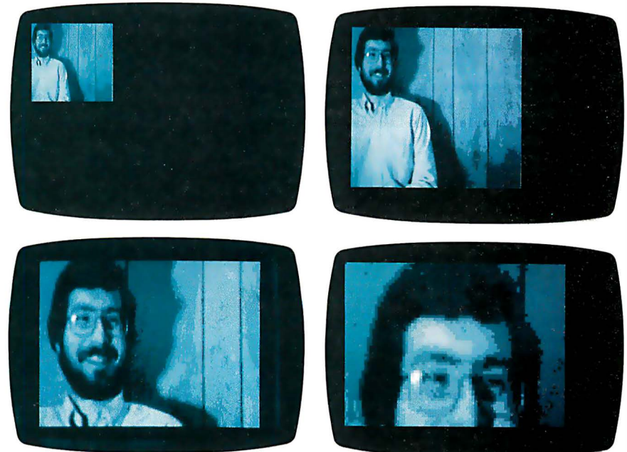
Photo 10: An image digitized on the ImageWise digitizer/transmitter is displayed on the GT180 (a). This image is magnified 2 times (b), 4 times (c), and 8 times (d).
