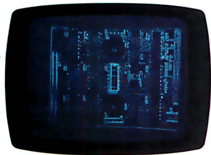
Photo 5c: The missing IC stands out.
