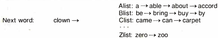
Figure 2: One individual list for each letter of the alphabet. Using 26 lists instead of one significantly reduces the average search time.
