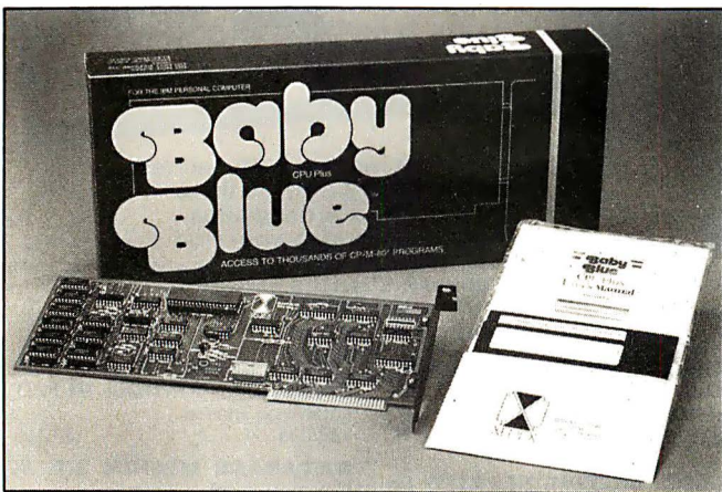
Photo 1: The Baby Blue CPU Plus from Xedex converts your CP/M-80 files into PC-DOS format and attaches a header to the file to identify it. You don't have to keep track of two different file formats.
