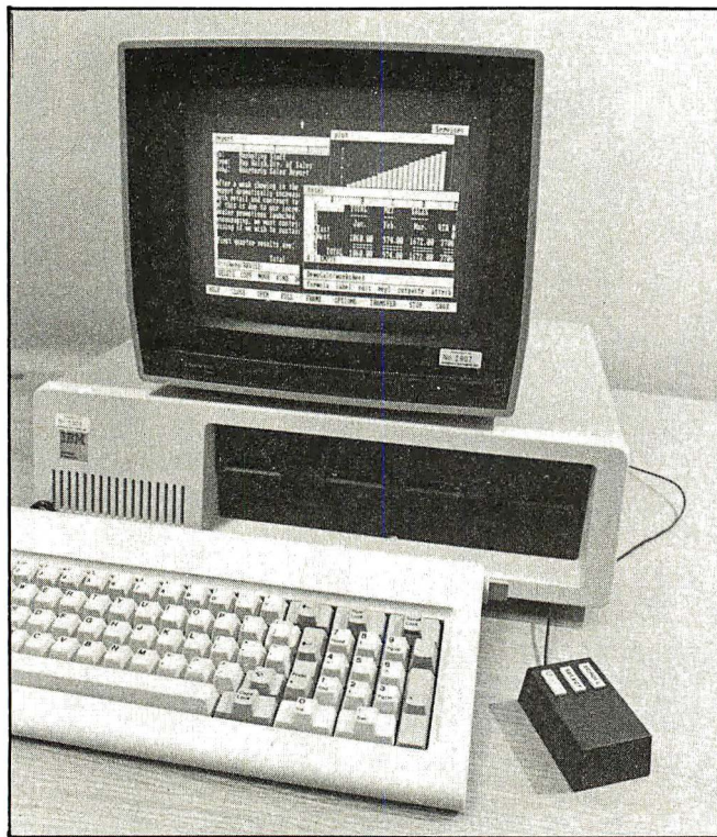
Prototype of Visicorp's Visi On integrated applications environment. Note the multiple video windows and mouse. Since this photo was taken, Visicorp has changed to a two-button mouse.
