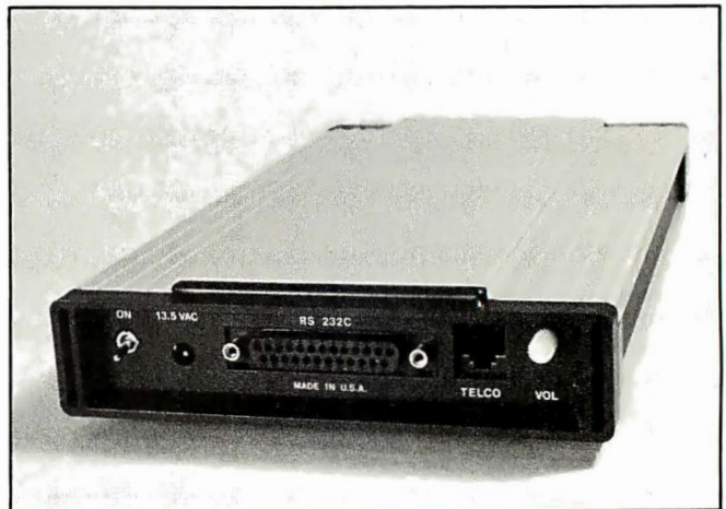
Photo 2: Front and rear views of the Smartmodem. In photo 2a, the seven LED status indicators are visible; photo 2b shows the power control, power connector, and RS-232C connector.
