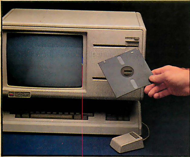
The Lisa floppy-disk drive, along with the special floppy disks it uses.
