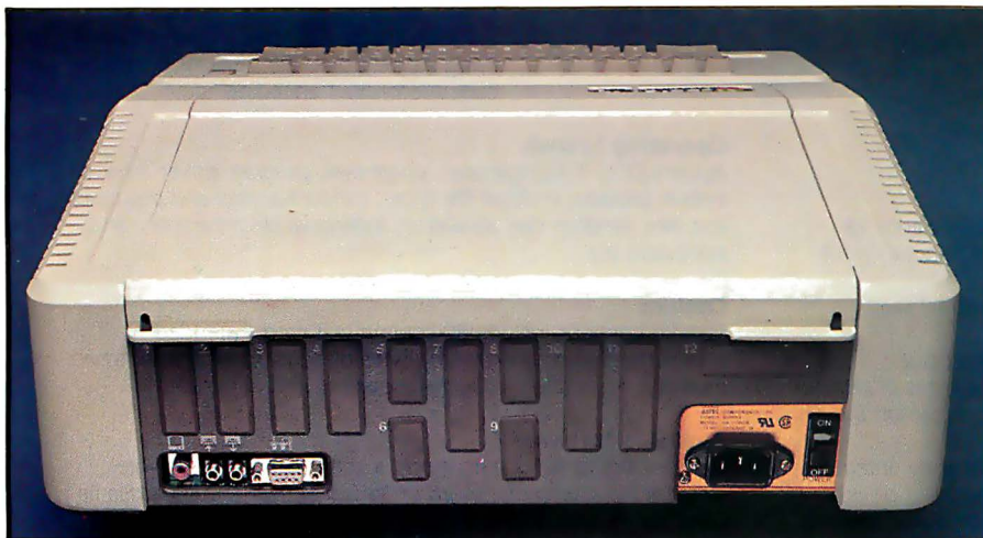
Photo 2: The rear panel of the Apple IIe. Instead of the plastic slots found in the Apple II, the Apple IIe's metal back panel is designed to mount 9-pin, 19-pin, and 25-pin D-type connectors in pre-cut recesses, providing more reliable connections and reduced RF interference. The built-in game-paddle connector has also been changed to a 9-pin D-type; however, the older-style connector is still available inside the case to accommodate existing devices.
