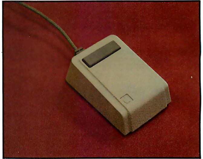
Photo 3: The "mouse" pointing device is about the size of a package of cigarettes and has one button on top.
