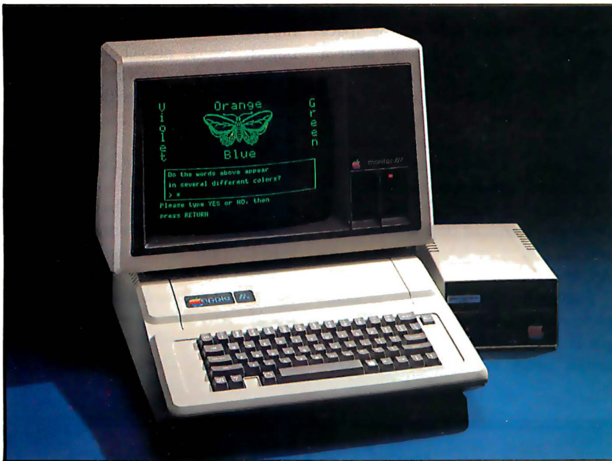
Photo 1: An Apple IIe system made up of the Apple Monitor III, the Apple IIe computer, and a Disk II 5 1/4-inch floppy-disk drive.
