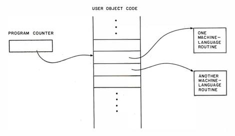
**Figure 1:** Simple threaded object code. The program counter points to certain object code, which in turn points to a machine-language routine. When that routine is finished, the program counter is incremented and points to the next object code, which points to the next machine-language routine.
