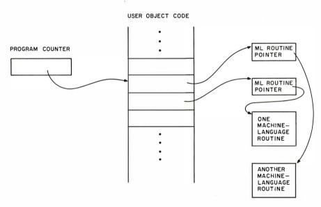
**Figure 2:** Threaded object code, FORTH style. In FORTH the object code points not to a machine-language routine, but to another pointer, which then points to the routine. If the routines are short, more time is spent jumping to the routines than executing them.
