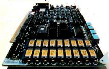
But that's not all. Each SLAVENET processor board comes with 128K of RAM, so a fully-populated Betasystem II has 1,088K of on-board RAM. Imagine, over a MEGABYTE of RAM, Run at peak system performance no matter how many users are on-line.
