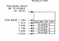
**Figure 2:** Memory allocation for the player-missile graphics. Definitions for the shape and vertical position of both the players and missiles are kept in this area of memory.
