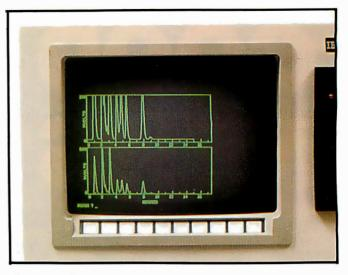
Photo 6: Close-up of the 12-inch, green-on-black raster-scan CRT display, with 768- by 480-pixel bit-mapped display and 80 characters by 30 rows. Ten user-definable keys are located along the bottom of the display, with user-chosen legends on the screen. The display has a unique single-lever tilt and swivel adjustment.
