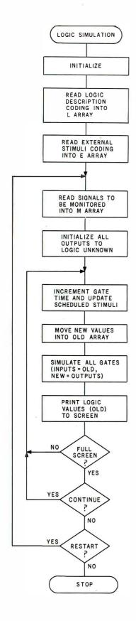
Figure 2: Flowchart of the Logic Simulator program. The simplicity of this diagram should lend encouragement to those interested in simulating digital logic circuitry. The implementation of this program in a high-level language (see listing 1) can be quite short.
