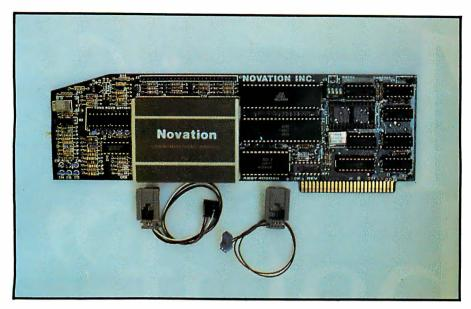
Photo 1: The Apple-Cat II basic system circuit board with the telephone connector cables. The cables are connected to pins located along the top of the card. Also shown are the two empty sockets for chips. The one on the left is for the Touch-Tone receiver chip; the other one (near the upper right corner) is for firmware ROM chips. (All photos are by the author.)
