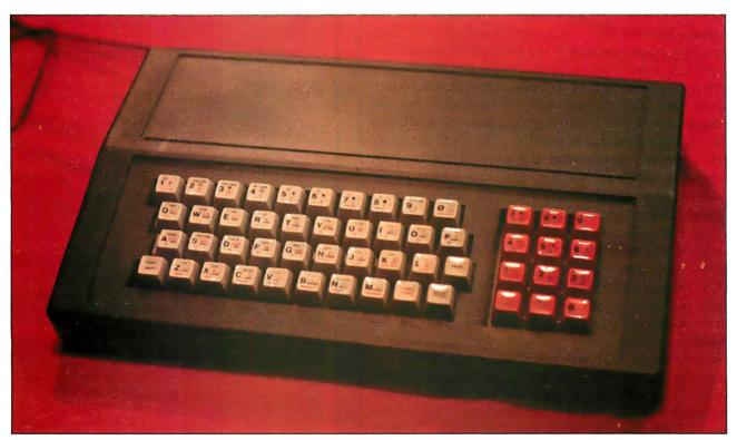
The Sinclair machines may be the most popular in Britain, but that doesn't mean that people like their keyboards—a brisk market exists for add-on keyboards and enclosures for Sinclair machines. This one, from DK'tronics, includes a full-size keyboard with keypad and an enclosure large enough to fit the computer board and other Sinclair peripherals. Its £45 price tag (almost as much as the £50 ZX81 computer) indicates the amount of interest in such products.
