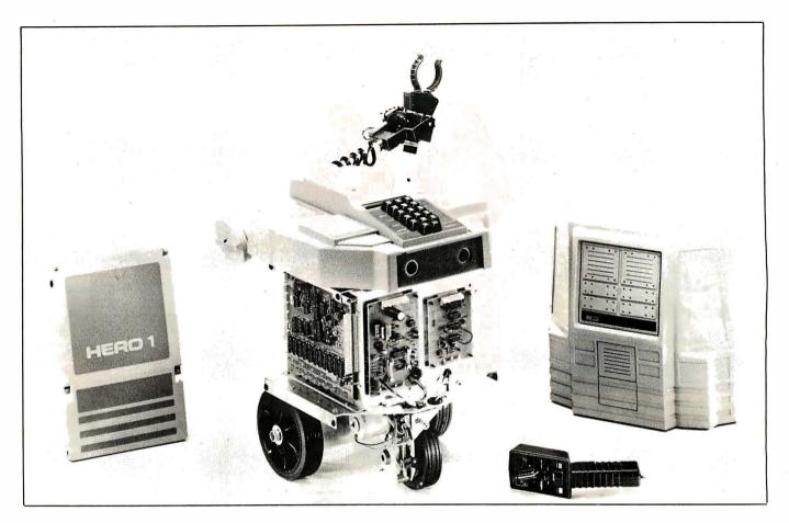
**Photo 2:** The Heath HERO-1 robot from the assembler's perspective. Note the teaching pendant (remote control) and the variety of sensors in the robot's head.
