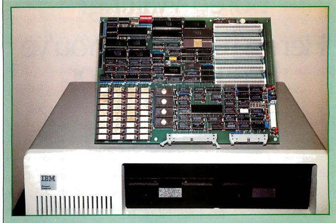
**Photo 1:** The MPX-16 has been designed to be compatible with the IBM Personal Computer in that peripheral devices made for use with the IBM PC can be plugged into the I/O-expansion bus of the MPX-16.
