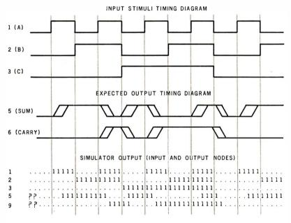
Figure 1: Example application of the simulator. The user provides a coded description of the electronic circuit (a full adder, shown at top), as well as a coded description of the input stimuli desired (in this case, the eight possibilities provided by three binary digits). The simulator produces a list of the binary values at each input and output. The user can then compare the list with the expected response. (A"." means logic 0, a "1" stands for logic 1, and a "?" means logic unknown.)
