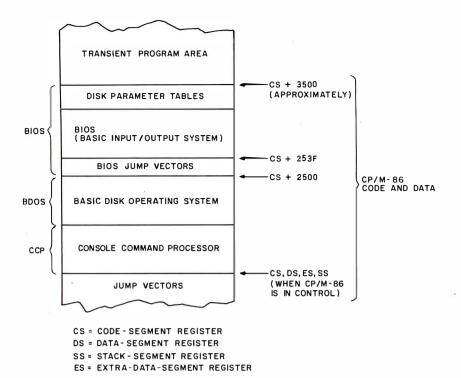
**Figure 3:** Memory map of the CP/M-86 operating system as configured for the MPX-16. In 64K-byte systems, the CS, DS, SS, and ES registers will all contain a value of zero, and the segments will overlap. User programs are loaded into the TPA (transient program area).
