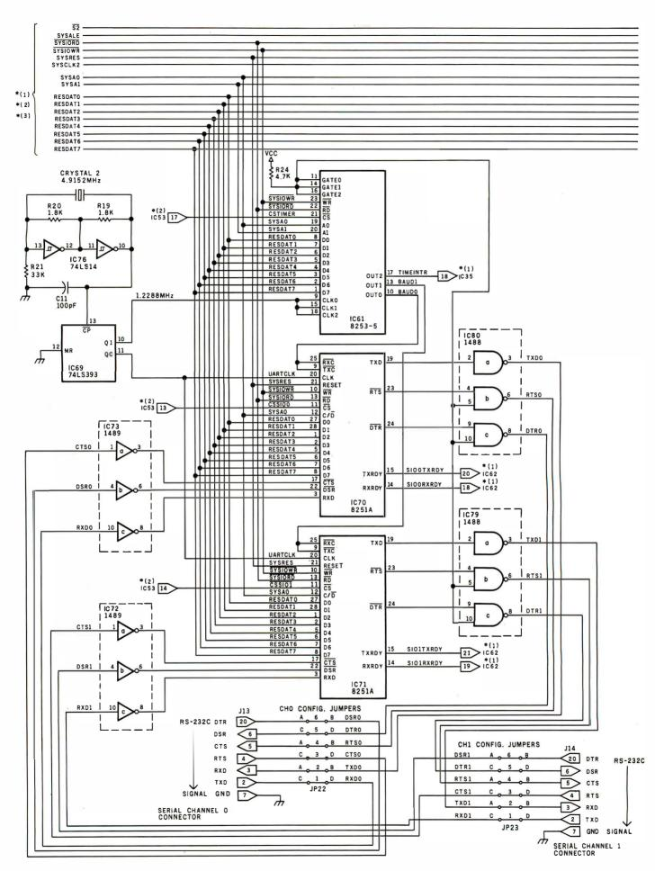
**Figure 1:** Section 4 of the schematic diagram of the MPX-16 computer. Section 1 appeared in November's article; sections 2 and 3 appeared in December's article. Connections to other sections of the schematic are shown by the notation \*(n), where n is the number of the other section.
