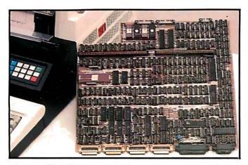
Photo 3: The IBM 9000 seven-layer planar processor board, showing the remarkably dense population of ICs and VLSIs. This state-of-the-art board has over 1600 test points and could not have been manufactured just over a year ago because of the density of the components. By plugging in an optional expansion board, up to five Versabus (a 32-bit bus standard developed by Motorola) cards can be plugged into the main board.
