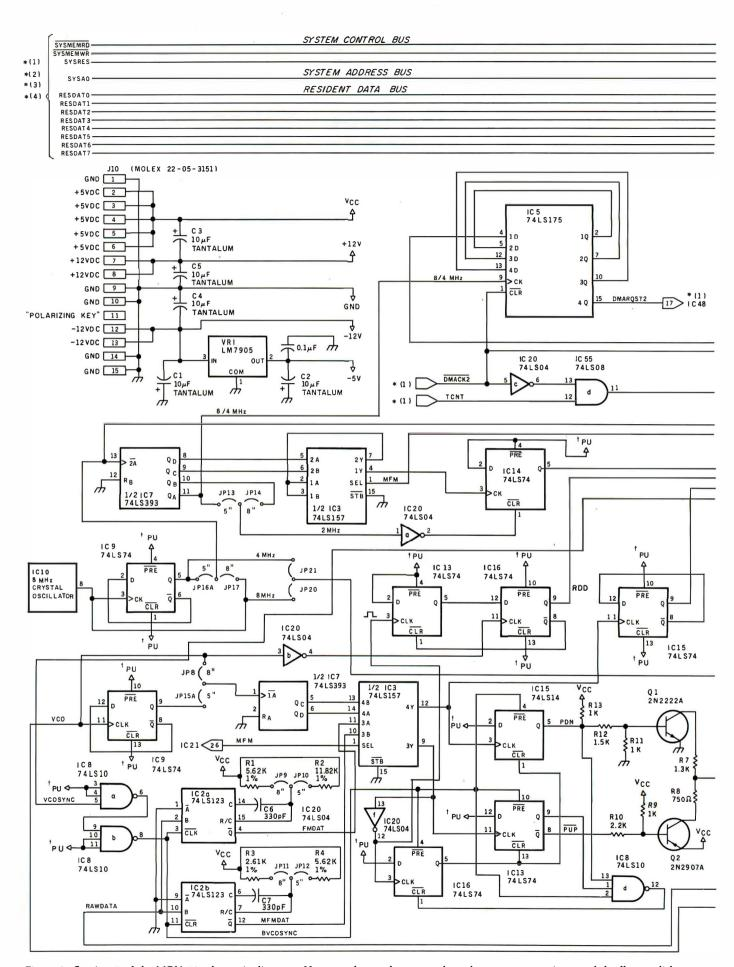
**Figure 2:** Section 5 of the MPX-16 schematic diagram. Here are shown the system-board power connections and the floppy-disk controller, including the PLL (phase-locked loop) circuitry used to recover data read from a disk. Connections for both 8-inch and 5¼-inch drives are shown.
