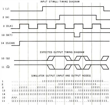
**Figure 3:** Simulation of the logic of a JK flip-flop. The design uses simple NAND and inverter gates and is presented to the simulator in the same way as in figure 1. The success of this model demonstrates the simulator's accuracy with sequential systems. (Crosscoupled gates used as latches present no problem.)
