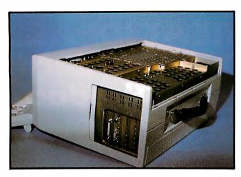
**Photo 4:** A second access panel covers the three expansion slots.
