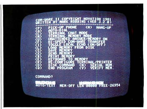
Photo 4: The main menu of Com-Ware II, the Apple-Cat II's terminal program, as shown on the author's screen. The two lines at the bottom form a status display. Commands are entered via a single keystroke. Pressing < ESC> in any mode will return you to this screen.
