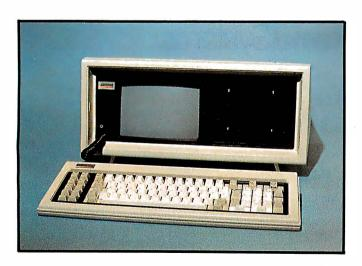
**Photo 1:** The Compaq computer is a portable system that is compatible with the IBM Personal Computer and less expensive.
