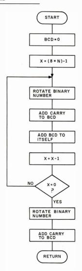
**Figure 1:** Flowchart of the binary to binary-coded-decimal (BCD) routine given in listing 1.
