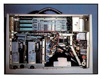
Photo 2: By removing the top, you can easily reach the circuit boards, video display, and power supply for servicing.
