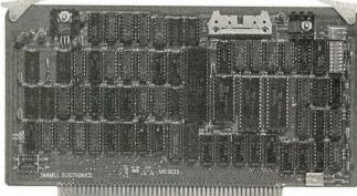
One of the outstanding features of this Tarbell CPU board is memory-management hardware that allows dynamic mapping of logical to 1 Megabyte of physical memory in 4K blocks. The on-board table memory may be loaded by the programmer or system software with I/O commands.
