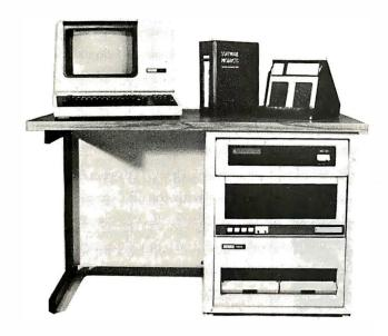
**CI-MWS03-SB** — LSI 11/2 computer workstation. LSI 11/2 CPU, 64KB Memory, power supply, KEV 11, in 16 slot rack mountable chassis. 2 port serial I/O. CRT terminal. 1 mega byte floppy disk system. Desk-
