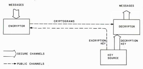
Figure 2: A public key cryptographic system. Encryption keys can be safely sent over the ordinary communication channel because the information they contain cannot be used to decrypt messages. Decryption keys are created near the decryptor and are not sent anywhere else. Each person who expects to receive encrypted messages creates a key for encryption and a corresponding key for decryption and sends the encryption key to those who will originate the messages.
