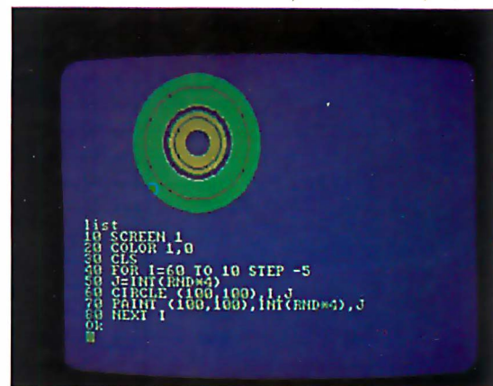
Photo 7: An example of combining text and graphics on the same video screen. The program shown, when run, generates the circular image just above it.
