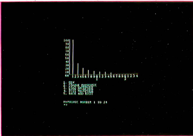
Photo 10: A plot of the harmonic partials required to create an approximate square wave. For each odd harmonic specified, the amplitude is equal to 100/n , where n is the harmonic number.
