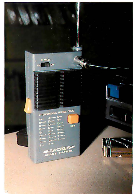
Photo 8: The output of the modem modulator is connected by a cable to this walkie-talkie (a Radio Shack number 60-4001) for transmission to the receiver on the Big Trak. The connection to the transmitter section of the walkie-talkie is made across the speaker terminals, with a 10-ohm resistor inserted in the circuit in place of the speaker. A phono jack installed on the front of the walkie-talkie facilitates the connection.
