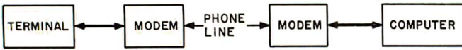
Figure 1: Diagram of a typical setup that allows a terminal to communicate with a computer over standard telephone lines. The modems shown are called DCE, or data-communication equipment, while both the terminal and the computer are called DTE, or data-terminal equipment. When referring to the RS-232C serial interface, the transmit/receive designation is always defined in terms of a DTE-to-DCE connection.
