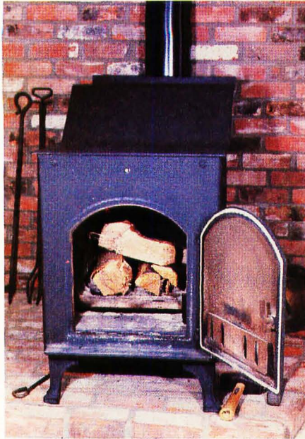
Photo 2: Logs up to 24 inches in length are placed in a grate which consists of water-filled tubes.
