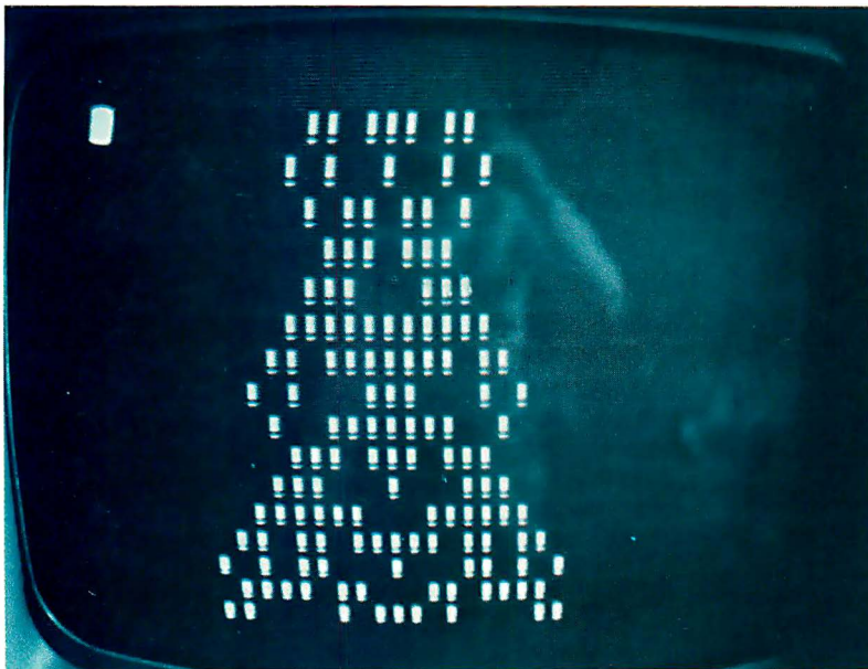
Photo 1: One-Dimensional Life display. On the author's system, 1s are represented by exclamation points and 0s by blanks. Each line represents one generation of One-Dimensional Life.
