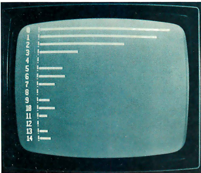
Photo 2: Video graphics display of the magnitude spectrum corresponding to the pulse shown in figure 4. The display is of course rotated 90° from the basic mathematical form illustrated in figure 2.
