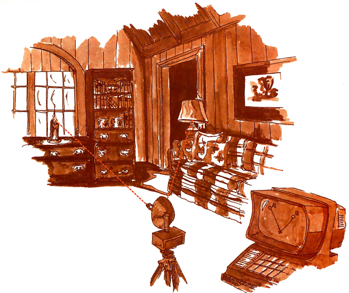
Circuit Cellar experimental setup showing the parabolic scanner as it detects a candle.
