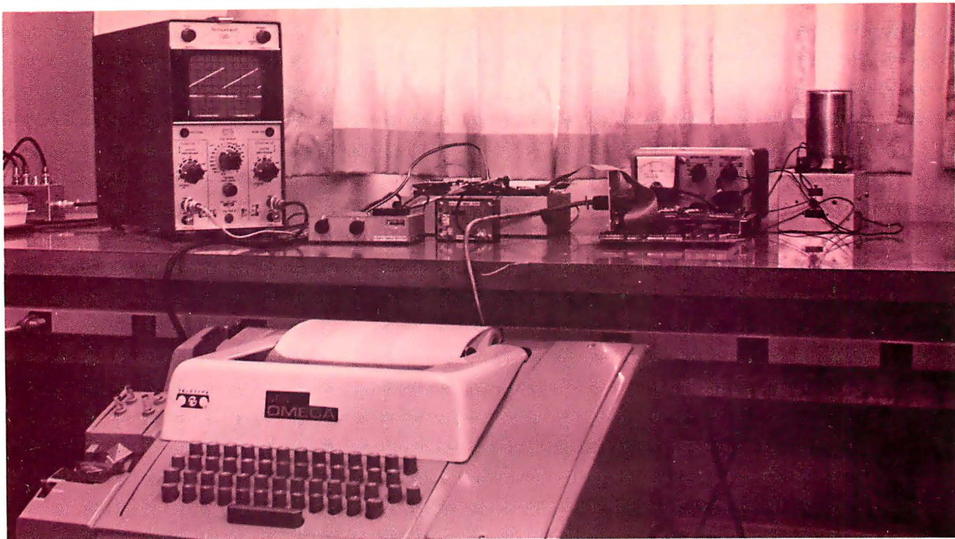
Photo 2: Mini-O in operation on the bench. The setup shown here uses a Teletype Model 33 ASR with the JOLT computer (at right in front of power supply), and the Sinclair clock reference (in front of interface box on bench). The display on the oscilloscope shows output from a lines of position digital to analog conversion output described (in concept) in part 1 of this article.
