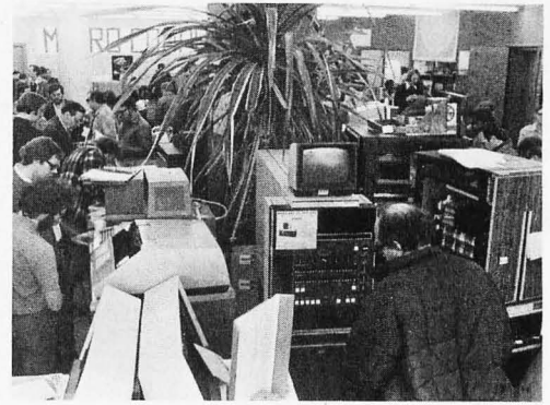
The maker of the potted palm is unknown, but computer-watchers will identify a rare Memorex MRX-40 (an IBM/360 Model 40 look-alike internally) under the palm, with an early DEC PDP-8 at the right. Since the Computer Warehouse store combines all the delights of a surplus house (it's the back side of American Used Computer) and a regular computer store, it is definitely a "must stop" on any computer hacker's tour of the Northeast.
