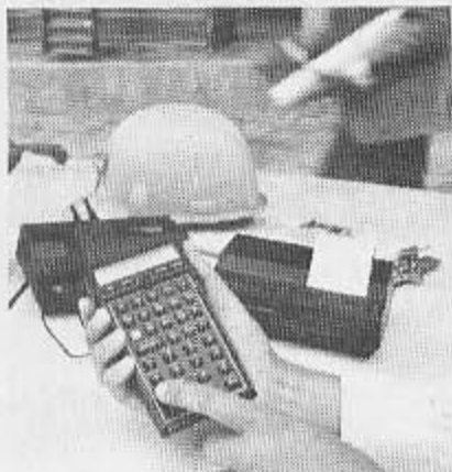
Series 40 Handheld Computers. They bridge the gap between calculators and desktops. And control up to 30 peripherals through the HP-IL interface loop.
