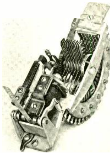
No. 359 Tool used for cleaning No. 200 type selector
