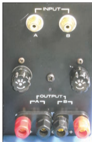
Photo 2: New in-out connection
