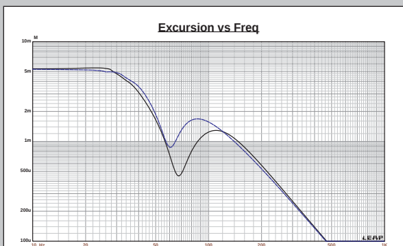
Figure 4: Cone excursion curves for the 7.5-V curves in Figure 3
