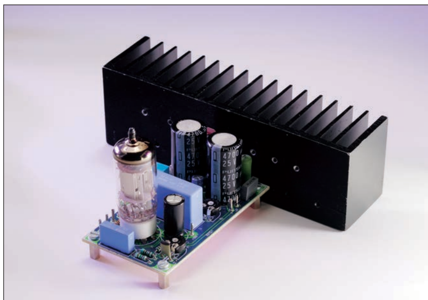
Photo 1: This simple amplifier uses a valve as a pre-amplifier and a MOSFET in the output stage.
