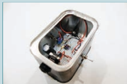
DIY Laser Audio Transmitter: "We wanted to see if it was feasible to transmit audio through use of a laser transmitter and a solar panel receiver. The laser transmission setup was connected to our development board and the solar panel was connected to our guitar amplifier. We managed to transmit pulse-width modulated signals from one floor of the house to another!"
