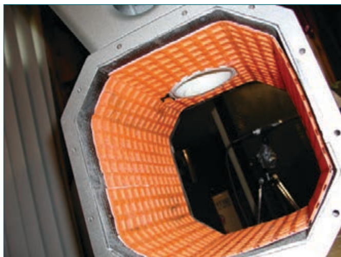
Photo 3: This is the woofer cabinet with 4" pipe leading to the 1.5" chrome vent tubes.
