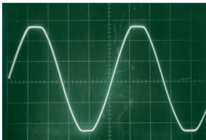
Photo 4: The clipping behavior at 11 W/1 kHz (5 V/div)
