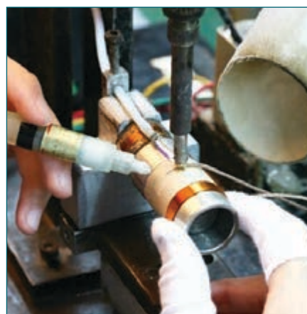
Photo 3: A voice coil goes through the winding process (Source: Po Yun Enterprise)
