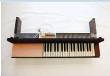
DIY SidCog Organ: "Whisker loves the SID Chip, the programmable sound chip of the Commodore 64, and all of the tunes it can make, and he also loves organs. So naturally he'd use the sound emulation properties of the chip with the form factor of an old Hammond organ! He's since added the ability to add release, sustain, echo, and decay before or during playing."
