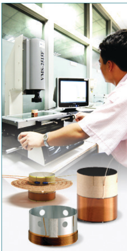
Photo 4: A worker inspects the voice coils (Source: Po Yun Enterprise)
