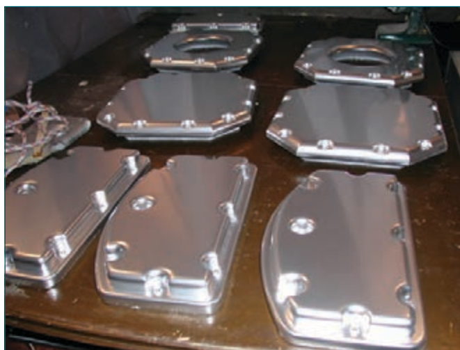
Photo 5: Sections of the speaker coated with Dupli Color chrome spray paint
