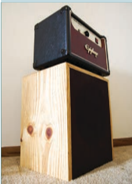
DIY Cabinet Speaker: "We have tons of instruments around and wanted a cheap and gritty way to listen to our jam sessions. So, we built our own cabinet speaker with cheap but functional pine and speaker. It sounds down-to-earth, the way we like it!"
