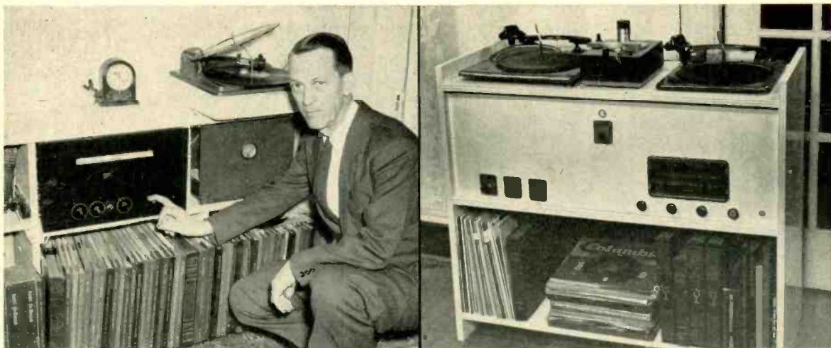
Left, the author at the controls of an early version of his home reproducing system. Right, later model of the system, with three changers for 78, 45, and 33 1/3 r.p.m. records.
