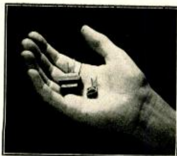
Fig. 5. Miniature compensating reactor and impedance matching transformer employed in the KB-2C microphone.
