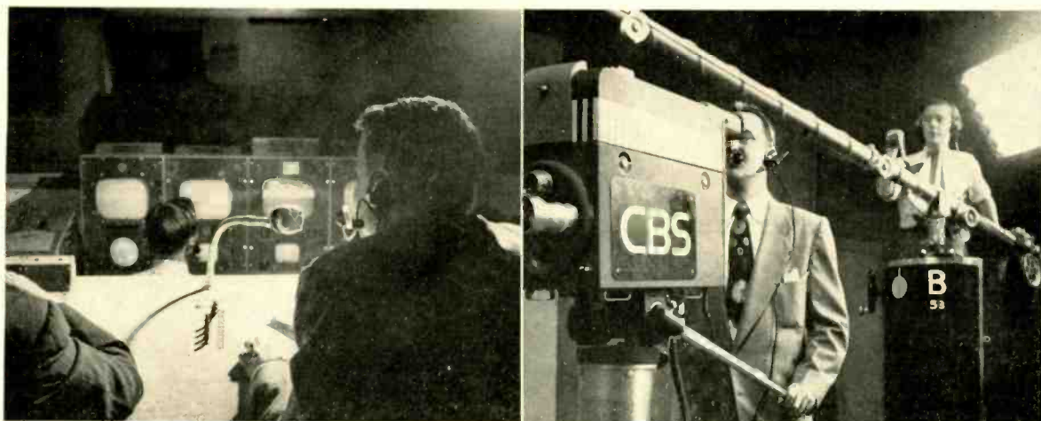
Fig. 1 (left). The director's position in a CBS-New York television studio. Four of the key switches on the small control panel connect the director's interphone instrument to various interphone stations in the studio. Two other key switches connect his desk microphone to the studio talkback loudspeaker and to the telecine room intercom loudspeaker. The assistant director is equipped with identical facilities. Fig. 3 (right). The type of telephone headset shown is generally used by CBS cameramen and camera control operators. The microphone boom operator in the background is wearing a pair of split headphones by means of which he receives instructions and cues.
