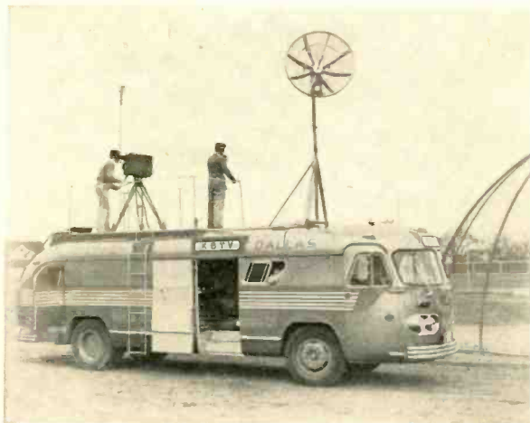
Fig. 1. The KBTW Telecruiser in use on location with the microwave relay "dish" in operation on its collapsible tower.
