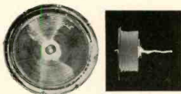
Fig. 12A (left). Cone breakup at 940 cps, with two radial nodes; point D. Fig. 12B (right). Transient response to same signal.
