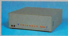
This state-of- the art 48MB 28ms lightning fast drive from Triangle comes with ROM autoboot for an extremely fast boot up time. The Turbo 3 can support SCSI and Atari access modes and is fully compatible with emulators like PC Ditto, Aladin and Spectre 128. Comes complete with instructions, built-in PSU and matching Atari case.
