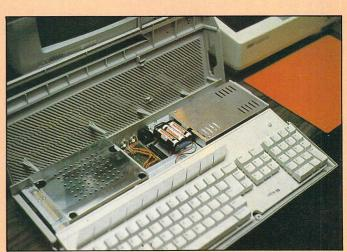
Fixing the battery in position with the sticky pad
