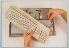
To remove the plastic cover, turn the ST over and remove the seven screws in the square holes. Lift the left side and manoeuvre the right side away from the disk drive. Then lift the keyboard and disconnect it from the computer.
