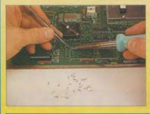
The hardest part involves de-soldering the legs from the motherboard. Make sure the soldering iron is hot and be careful not to overheat the circuit board. A solder sucker is essential. As each leg is carefully removed, you should be able see through the hole.
