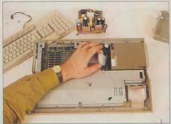
Junclip the power supply connector, remove the screws that hold the power supply down and move it to a safe place. The disk drive also needs to be disconnected; turn over and remove the three long screws in the round holes.
