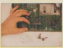
From now on it's plain sailing. Insert the socket provided with the installation kit and solder it into place. As before be careful not to apply too much pressure or heat on the main board and make sure that you don't solder two pins together accidentally.
