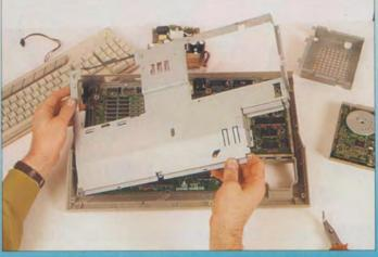
Once the disk drive and power supply unit are out of the way, the main metal screen can be removed. Straighten the metal twists but be careful – this can be a little fiddly. Also watch your fingers as the metal is quite sharp!
