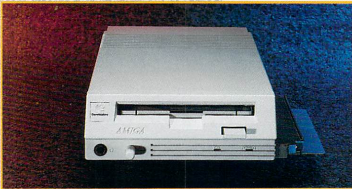
The headphone jack and volume control on the A570's front panel let you listen to audio CDs while working at your computer.
