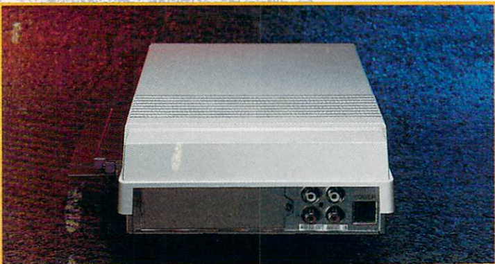
The route to A570 expansion is through the rear panel to the left of the audio jacks.
