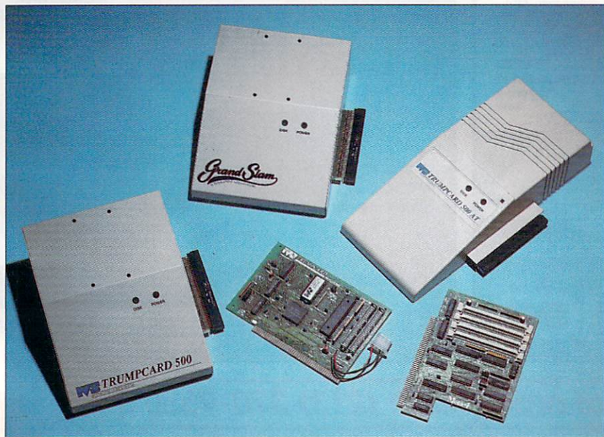
The IVS line of hard disks and RAM expansion for the A500.
