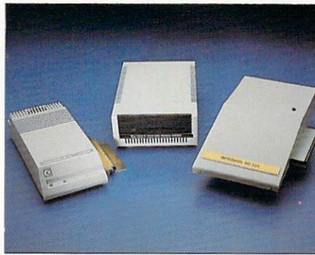
Drives in a row: (l to r) the A590, The Vault, and the HD-500.
