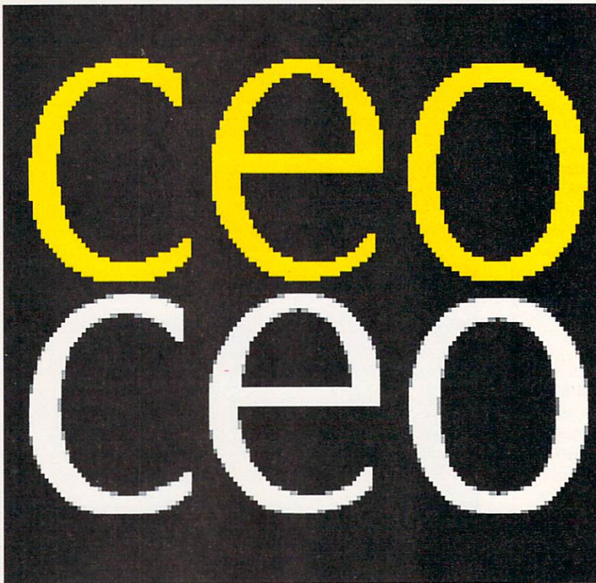
In normal resolutions, edges appear jagged (top); Broadcast Titler's super hi-res mode (bottom) smooths them.
