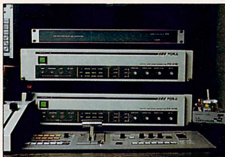
High-powered productions benefit from high-powered equipment. From left: a Time-Base Controller, an Edit Controller, and a Single-Frame Animation Controller.
