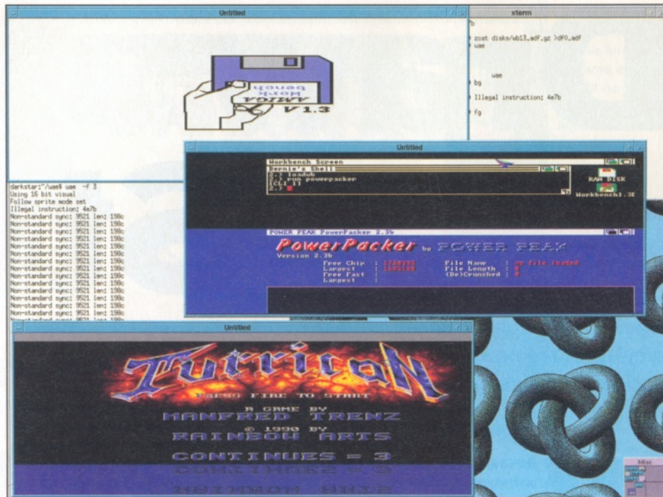
UAE can use any ROM image and so you can have a 1.3 machine, a 2.0 machine or a 3.0 machine depending on which Amiga you take your ROM from.
