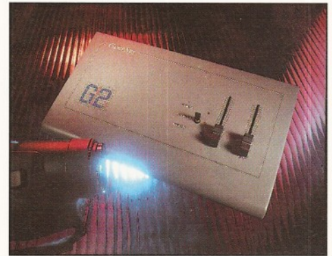
As the difference in price suggests, the G2 Systems Genesys outputs a higher quality signal than its VC1 stable mate; both composite and Y/C.
