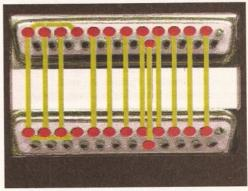
17-Bit Software's disk 2763 provides help on setting up Parnet, including diagrams like this.
