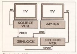
The Amiga's RGB output is connected to the RocGen Plus as can be seen above.
