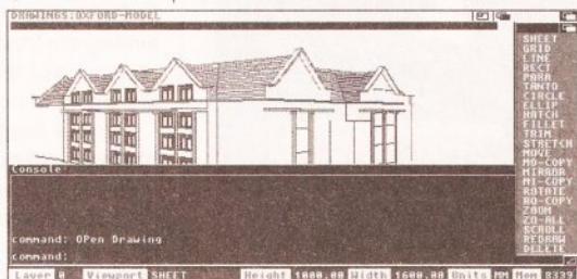
Although it may look 3D, this is a 2D perspective view of a 2D model, with hidden lines nicely removed.
