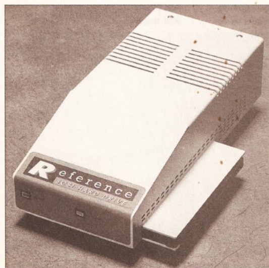
The Reference hard drive for the A500 – it's tough but noisy, and the external "dumb" PSU is troublesome.
