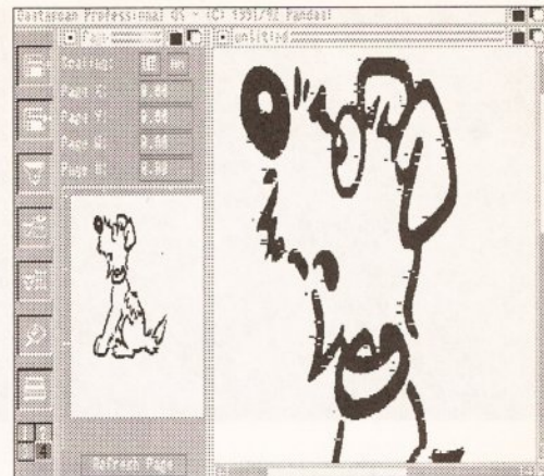
The DaataScan scanner corrupts 400 dpi line art scans with short horizontal black and white lines, however at 300 dpi and below scans are glitch free
