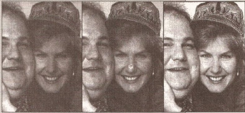
The results of converting a scanned halftone to 16 true grey levels; to the left is AlfaScan Plus, in the middle DaataScan and on the right Power Scanner
