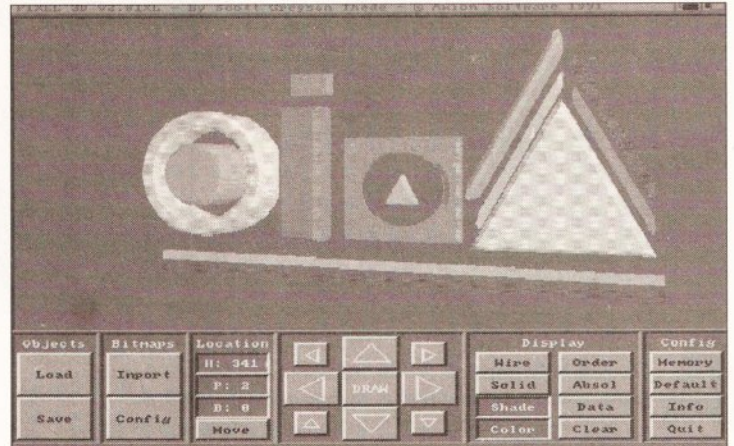
The results of extruding a bitmap image. Each colour of the image is set to extrude to a different length
