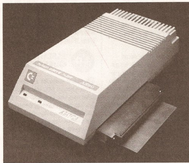
Commodore A 590 – despite lacking in RAM expansion, the controller is nigh on perfect. It looks pretty neat too, as the colour and shape are specifically designed to fit your Amiga
