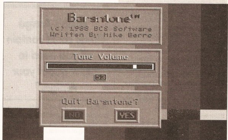
Barsitone , from PD Soft disk V518 is just one of the video tools available. It generates an industry-standard display and audio tone, for recording on to video tape as a 'leader'
