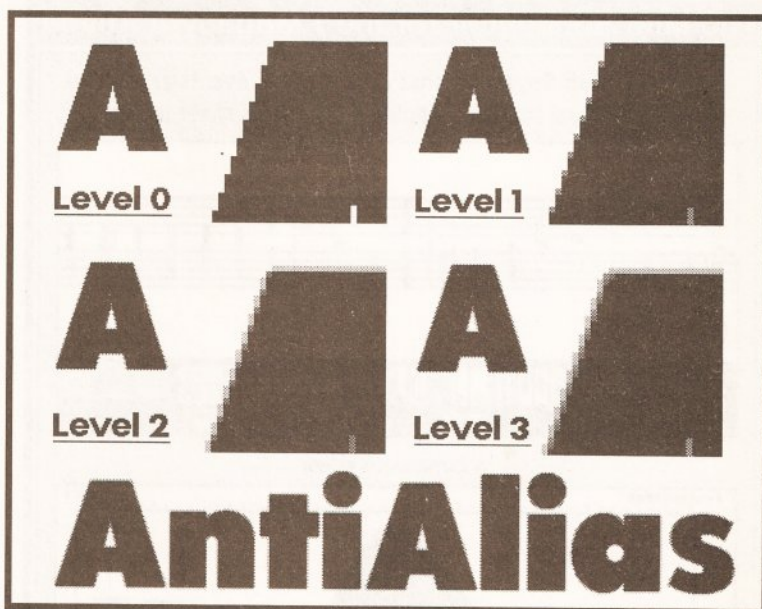
The three levels of antialiasing now available in Scala 1.1 . The edges of bitmap images (including text) are progressively built up with lighter tones to give a smoother appearance.
