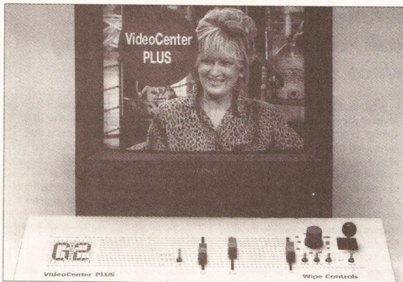
A genlock like this one from G2 Systems allows you to combine video with your Amiga's output to create a range of fascinating effects.
