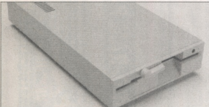
For those with 5.25" disks, Roctec's RF542 is a handy gadget, apart from the rather dippy DIP-switch drive disable.
