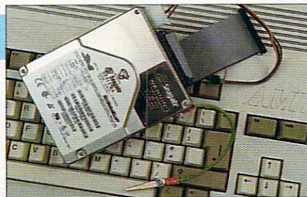
Most recent 3.5" hard drives should work without a problem in a 1200, as long as you have a fixing kit
