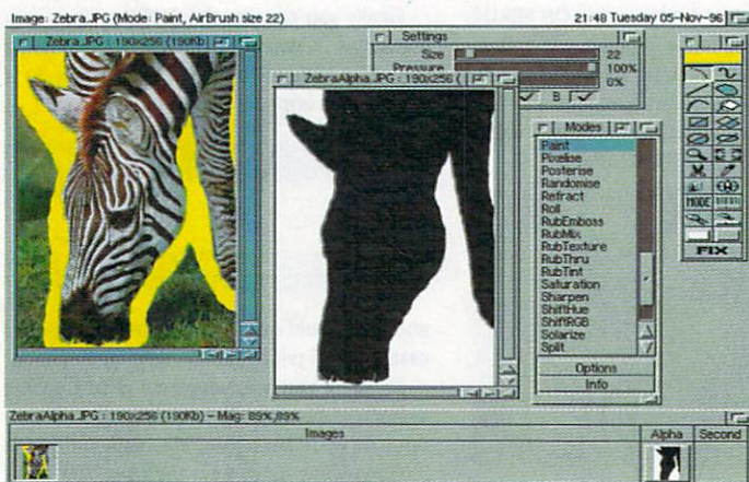
As the alpha channel has 256 levels you can use it to blend effects onto an image
