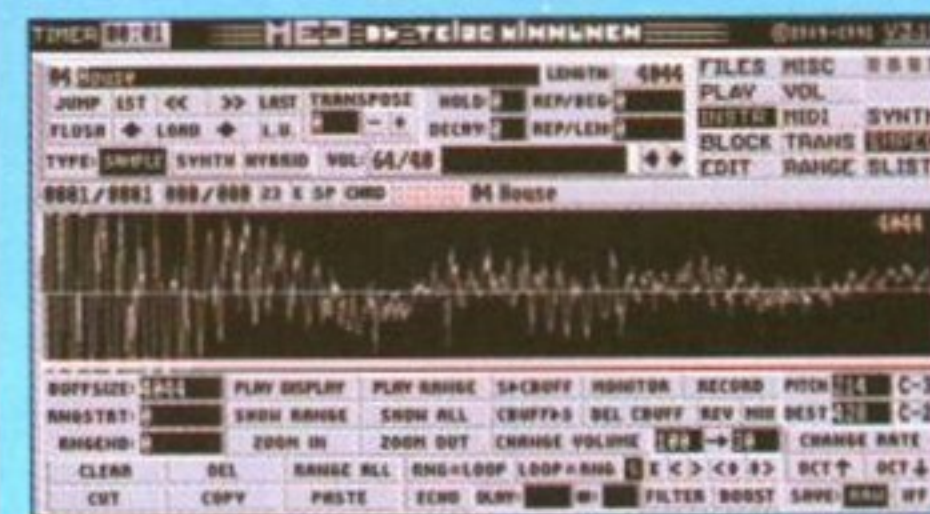
This is that same snare drum sound, but now it fades out towards the end. One way to achieve this effect, would have been to just ramp the volume down at the end of the original sample, but then you'd end up with a very short sound. Instead the sound has been lengthened a little, by echoing the second half, and then faded out.
