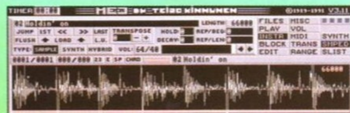
This one on the other hand, taken from the Soul II Soul track Holding On, is well suited to a bit of cutting and pasting. Notice the pronounced peaks and troughs, which mark the start and finish of each sound in the beat.
