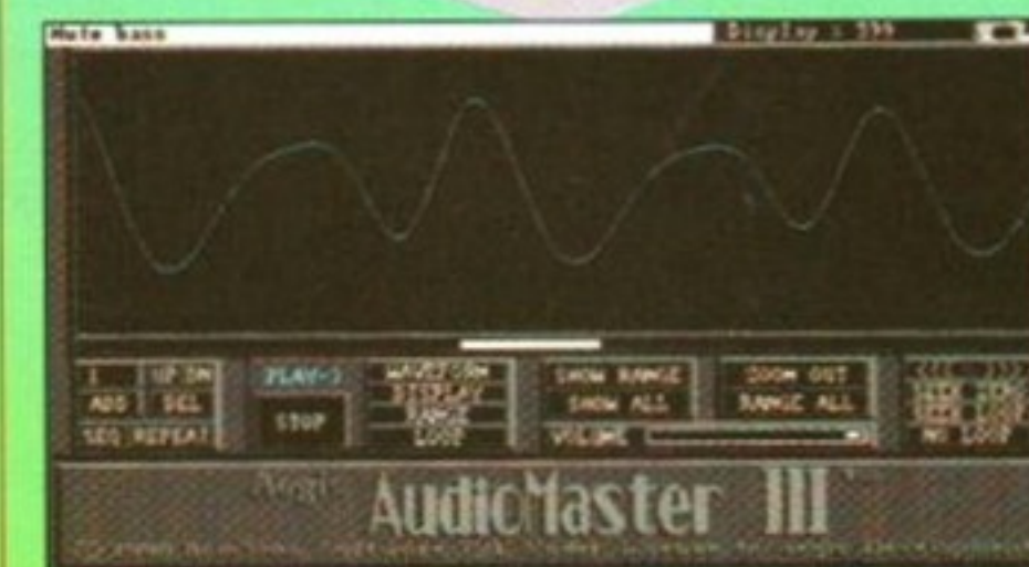
Looping can be used to great effect, giving your sounds an infinite length without using loads of memory. Finding suitable loop point however, can be tricky. Some sounds are impossible to loop in their raw state. The waveform of a synth sound, or a sampled trumpet for example, may never go "full circle", so it would seem that there's sometimes no alternative to an audible click on the loop point. Here's a quick trick that can be used to rectify the problem, and it works extremely well.
